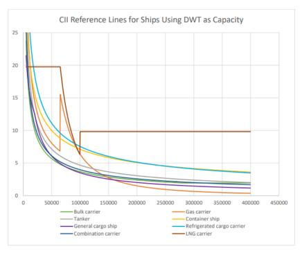
Figure 2: CII reference lines for different ship types
