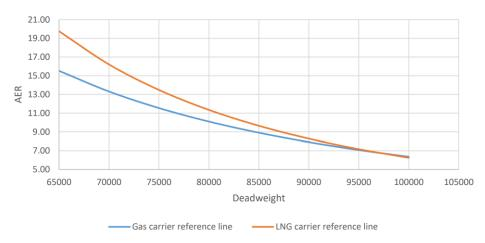
Figure 3: Comparison of LNG carriers in the gas carrier and LNG carrier CII reference lines between 65,000 and 100,000 DWT
