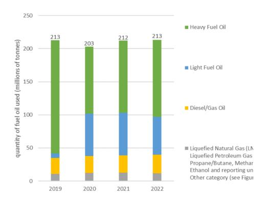
Figure 1: The aggregated annual amount of each type of fuel oil consumed ships of 5,000 GT and above from 2019 to 2022
