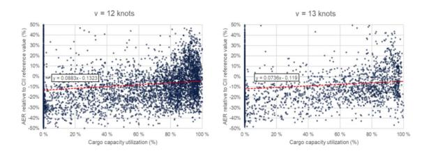
Figure 5: CII performance vs. cargo capacity utilization for each voyage, average speeds of 12 and 13 knots
